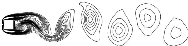
Fig. 1 Visualization of the instantaneous vorticity magnitude about the single square cylinder (case 3) at Re = 150 and tU_\infty/D = 400 with 20 equally spaced contours of instantaneous vorticity magnitude over the range 0.2 \leq |\Omega|D/U_\infty \leq 4 .
